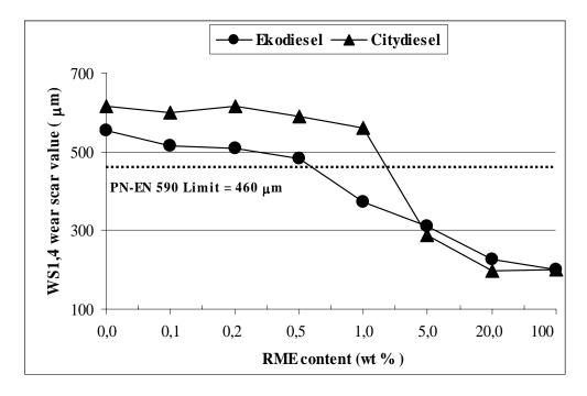
Fig. 2. Impact of the rapeseed methyl ester (RME) content on the HFRR lubricity of the Ecodiesel and Citydiesel diesel fuels
